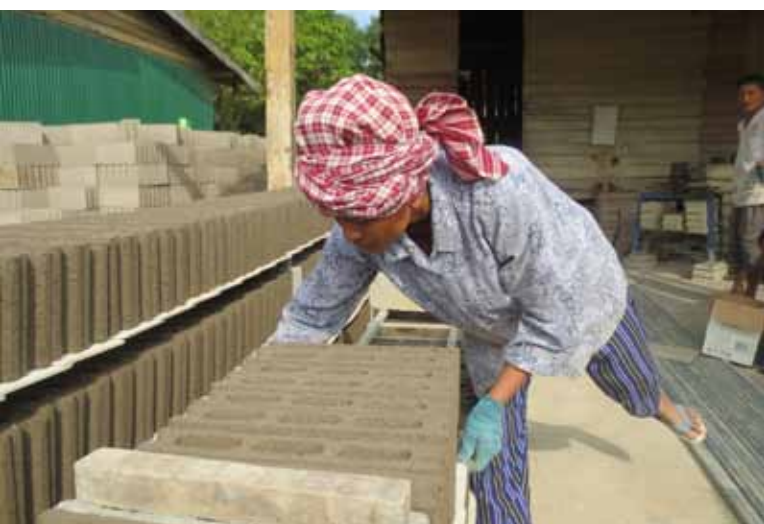
Small concrete brick production in Banteay Meanchey province.
